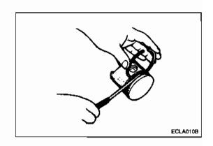
3. Measure the clearance between piston ring and ring home.
