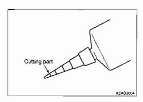
3. Squeeze the liquefied gasket from the tube and apply it to the oil pan as shown in the illustration.
