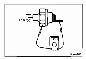
Apply a 0.5 kg/cm² pressure to the oil hole. The switch is normal if there is no continuity. Also check for air leaks. If any air leaks are detected, the cause may be a broken diaphragm. Replace the switch if it leaks.
