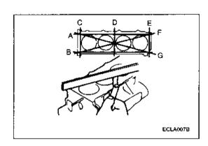
Using cylinder gauge, measure the cylinder bore. If it wears out excessively, bore the cylinder to oversize and replace the piston and piston rings. Measurement points are as shown.
