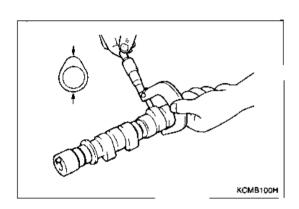
Check the cam surface for abnormal wear or damage and replace it if required.
