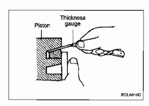
Place a piston ring in the cylinder bore and set it square by pushing it down with piston.
