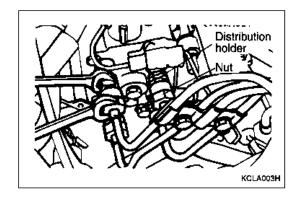
Loosen the injection pump mounting nut and temporarily tighten it.
