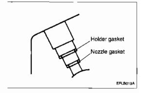
2. Fit a new nozzle gasket and holder gasket into the nozzle holder hole in the cylinder head.
