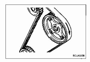
4. The piston in No. 1 cylinder is at the top dead center on the compression stroke when all timing marks at the three places are aligned as shown.
