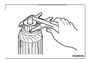
3. Check the depth of the undercut between segments.
