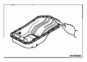
Cut the nozzle attached to the liquefied gasket as shown in the illustration. The liquefied gasket comes out with 4mm diameter.
