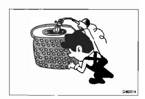
4. When the element is cleaned, remove the baffle and clean the dust cup, too.
