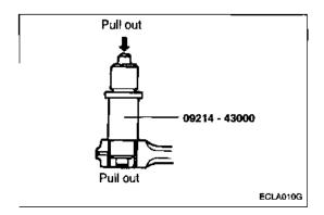
2.. Press-fit the bushing using the special tool.
