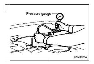
4. Crank the engine and measure the pressure.
