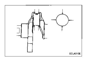
Measure the connecting rod bearing I.D. and crankshaft pin O.D. If the clearance (oil clearance) exceeds the limit, replace the bearing and, if necessary, the crankshaft. Or, grind the crankshaft to an undersize and, at the same time, replace the bearing with an undersize.
