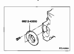
Using Bearing Installer Stopper and Silent Shaft Bearing Puller (09212 - 43300, 09212 - 43100), remove two rear bearings from the cylinder block.
