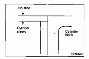
Chamfer the cylinder sleeve top end as shown in the illustration.
