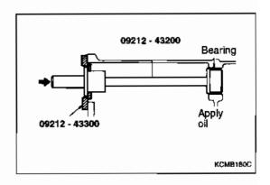
4. When press-fitting the right bearing, align the bearing oil hole with the cylinder block oil hole.
