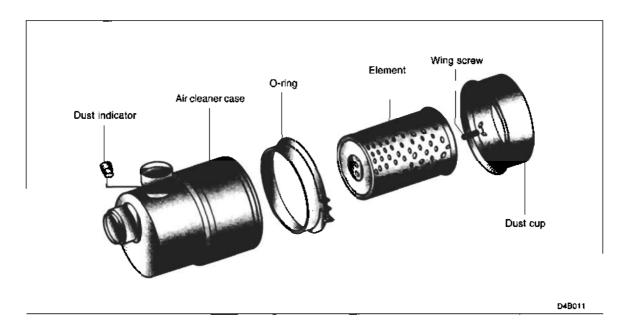
1. If the element is contaminated with dry dust, clean dust, etc. by blowing clean compressed air[685kPa(7kgf/cm²) or less] along the frills from inside the element.
