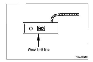
Unsolder the brush lead wires, and the brush and spring will come out.
