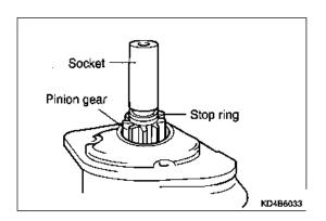
Remove the snap ring with a screwdriver, then, remove the stop ring.
