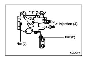
4. Remove the timing check plug from the injection pump.
