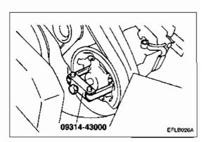
Leave the sprocket in the timing belt lower cover with the timing belt engaged.
