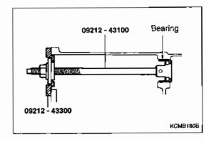
Using Bearing Installer Stopper and Silent Shaft Bearing Puller (09212 - 43300, 09212 - 43100), remove two rear bearings from the cylinder block.
