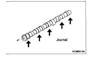
Measure the camshaft diameter and bearing inner diameter and if the oil clearance exceeds the limit value, replace the camshaft, cylinder head or both.
