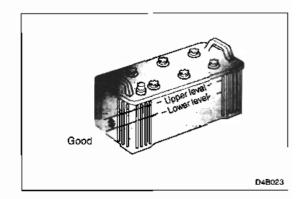
2. As for a battery which has no level lines, the level should be 10 to 15 above the battery plates. Add fluid until the fluid level reaches the lower surface of the case.
