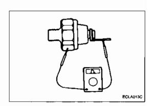
2. Insert a thin rod in the oil hole of the switch and push it in lightly. The switch is normal if no continuity is detected (infinite resistance on the tester). If there is continuity, replace the switch.
