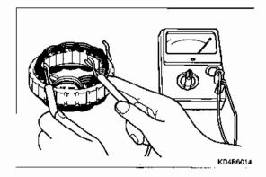
Check the coil grounding. Make sure that there is no continuity between the coil and core. Replace the stator assembly if there is continuity.
