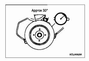
Rotate the crankshaft to the right to place the pulley notch to 5°.
