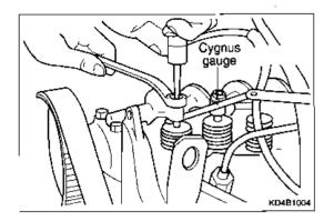
Measure valve clearance at arrow positions shown in the illustration.
