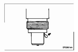
If there is leakage, disassemble injection nozzle and replace nozzle tip or entire assembly.
