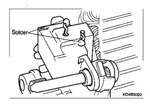
When installing a new brush, push the brush into the holder as illustrated and solder the leads.
