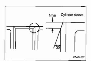
6) Cylinder sleeve I.D. is processed with 90.08~90.10mm, after press-fitting the sleeve, hone the bore to be within the standard value.
