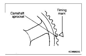
2. Adjust the valve clearance at the arrow position shown in the illustration.
