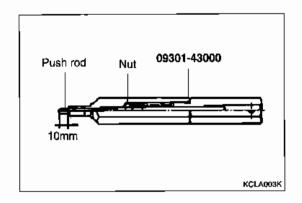
Install the dial gauge by installing the special tool to the injection pump.
