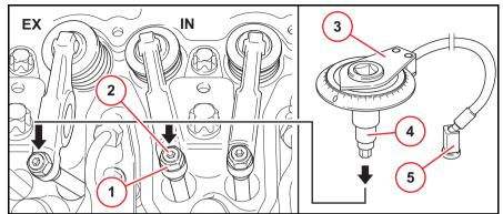
Set valve clearance (inner exhaust recirculation)
