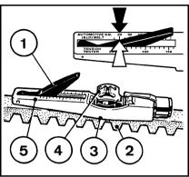
Checking the belt tension
