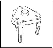
Special wrench for loosening exchangeable filters
