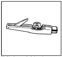
V-belt tension measuring instrument
