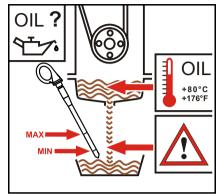
Checking the lubricating oil level
