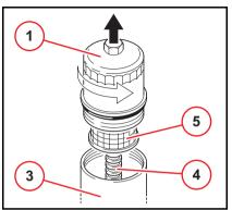
Replace lubricating oil filter cartridge
