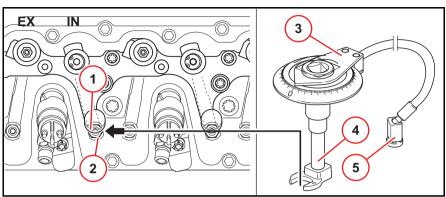
Set valve clearance (with internal exhaust gas recirculation EGR connected)
