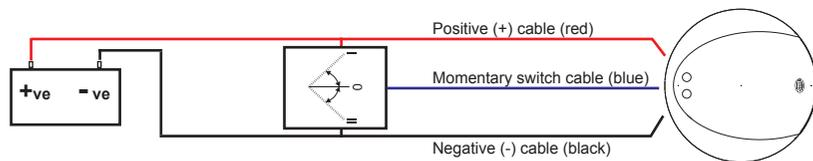
**Note:** Operation of the dimming function with an external switch will synchronise all lamps first before dimming
