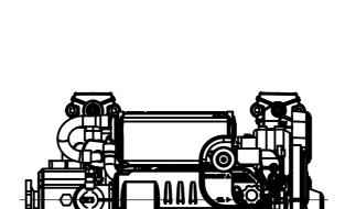
FUEL SUPPLY: 8 mm FUEL RETURN: 8 mm EXHAUST 40 mm SEAWATER INTAKE 20 mm
