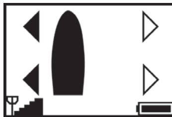
Bow and stern thrusters to port.
