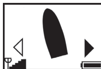
Stern thrusting to starboard.
