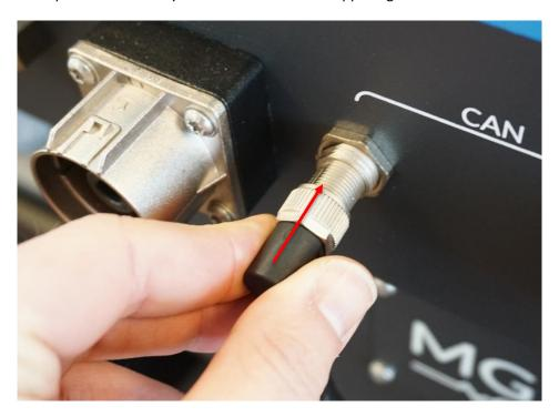
3. Lock the connector by rotating the locking nut clockwise. Hand-tightened will be sufficient, do not use tooling to tighten.
