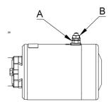
Motor Cable connections When tightening the cables to the motor, ensure the lower nut (A) is secure against turning when tightening the upper nut (B). This will prevent damage occurring within the motor
