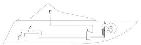
Solenoid pack (Required and included) The solenoid pack (B) should be located in a dry area close to the drum winch.
